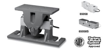
This product is designed to simplify the installation of the 65058 load cell into a certified Legal-for-Trade high capacity weigh bridge. Unilink™ floating suspension allows controlled floating of the scale deck, providing a reliable and accurate weighing system. The load cell is nickel plated or stainless steel and sealed to IP67 standards, assuring reliability. The mount assembly is provided with a primer coat finish to simplify the manufacture of the scale.
